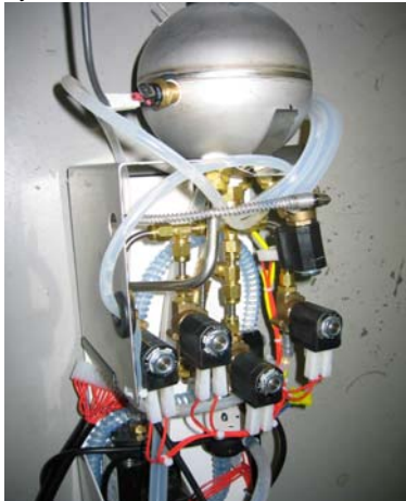
Boiler unit in the coffee machine ES 5100, SERTO unions join the media-conveying lines with the espresso module
